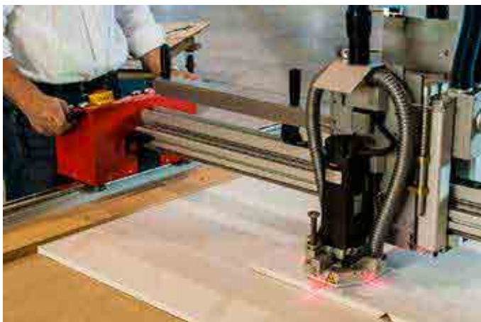
Rout assembly with the PanelMax panel fabrication machine
