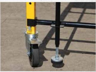
Each locking assembly must located on opposite corners of the scaffold.
